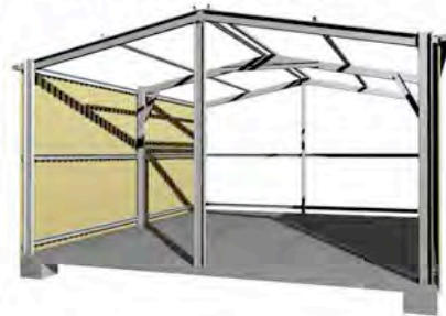
GABLE END WALL GIRTS IN PLACE
