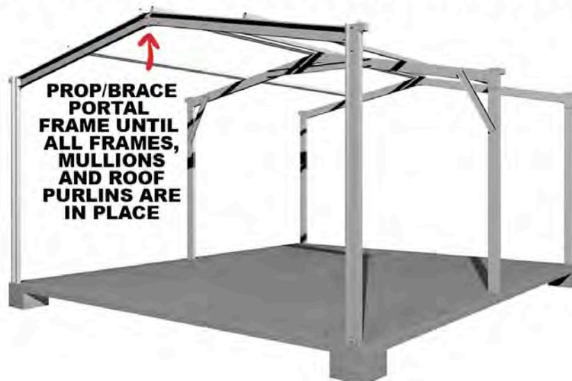
**Note:** Care must be taken not to allow rafters to rotate around haunch brackets. Use propping or extra roof purlins to achieve this.
