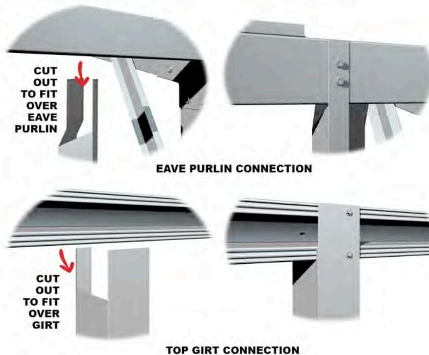
A Base Cleat Bracket is attached to the bottom of Each Side Wall Roller Door Jamb. Fit L/H and R/H side doorjamb and screw the two upright (uncut) legs to both sides of the SIDE WALL GIRT ABOVE or EAVE PURLIN using Framing Screws. Plumb the jamb and drill holes in the base cleat and anchor bolt into position. Fix the door jambs at intersection of any girt(s) which were cut off.
