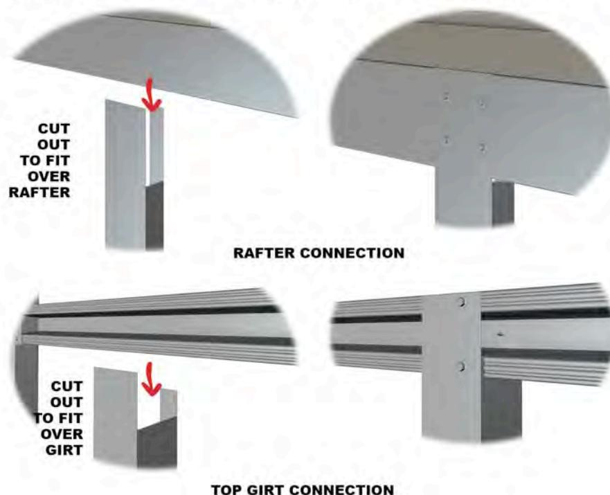
Measure the height of the GABLE END WALL GIRT BELOW and cut this amount out of the centre section of the bottom end of each Side Wall Roller Door Jamb as shown . If the Jamb sits on the slab then a Base Cleat Bracket is attached to the bottom of Each Side Wall Roller Door Jamb as shown.
