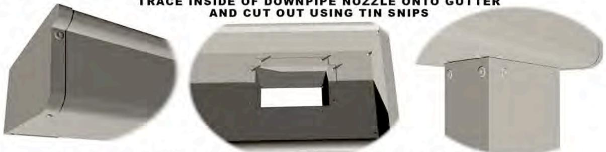
**ATTACH STOP ENDS AND DOWNPIPE NOZZLE WITH SILICONE & RIVETS**
