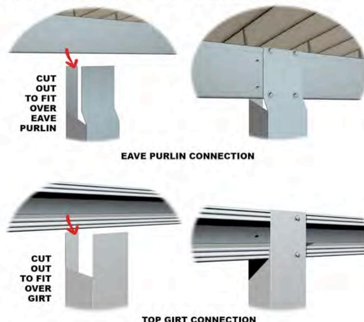
Measure the height of the SIDE WALL GIRT BELOW and cut this amount out of the centre section of the bottom end of each Side Wall Roller Door Jamb as shown.
