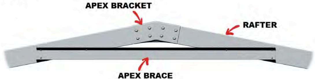
**Note: Under NO circumstances are the Apex Braces to be fitted to the lips of the C Section.**
