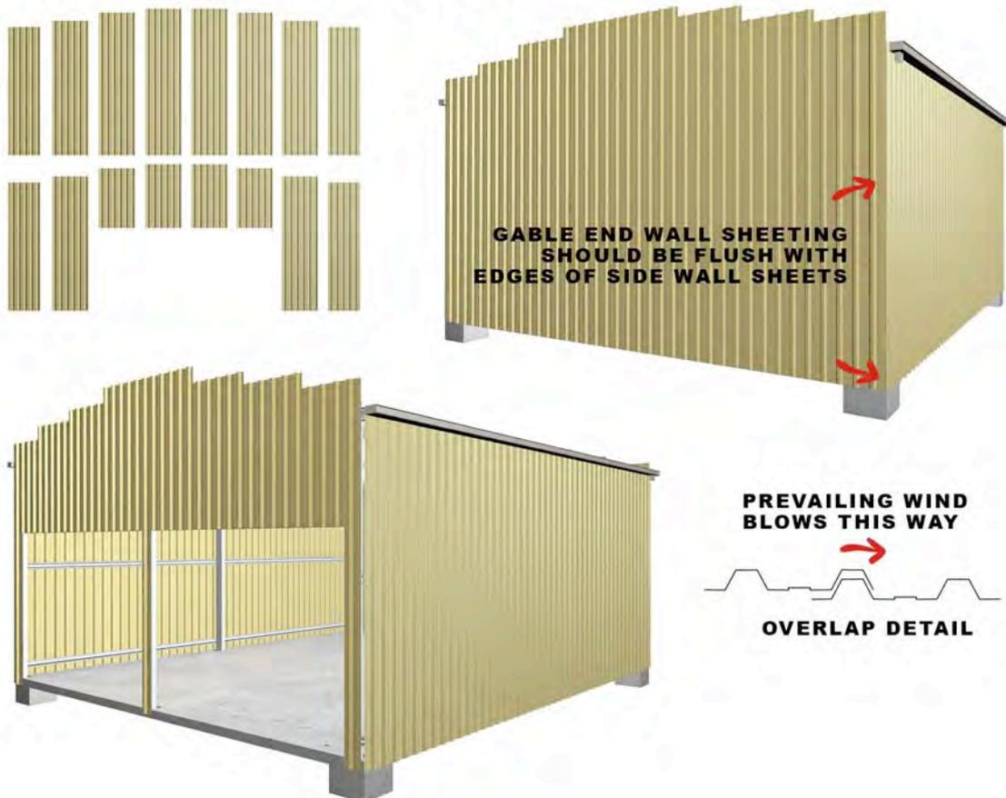
Once all the sheets are in position, trim the tops of the Gable End Wall sheets flush with the roof sheets using an electric nibbler or tin snips. Screw the top of the Gable End Wall sheets to the top lip of rafters.
